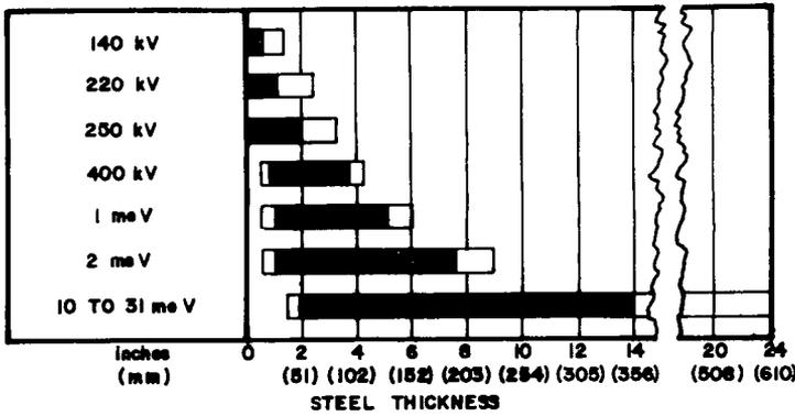
FIG. 1—APPROXIMATE PRACTICAL THICKNESS RANGES OF STEEL FOR VARIOUS X-RAY KILOVOLTAGES
