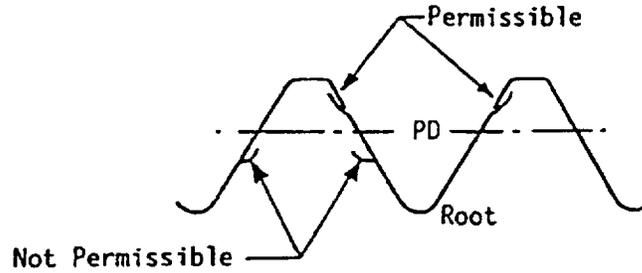
FIGURE 5 - Laps Extending Towards Crest, Rolled Thread
