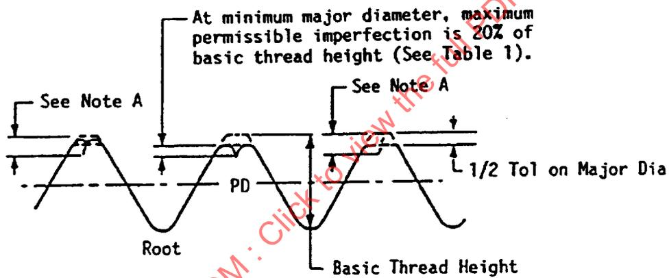
Note A: Maximum depth of imperfection equals 20% of basic thread height plus 1/2 the difference of the actual major diameter and minimum major diameter.
