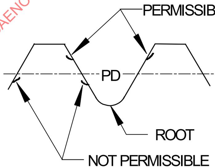
Figure 6 - Laps extending towards crest, rolled thread
