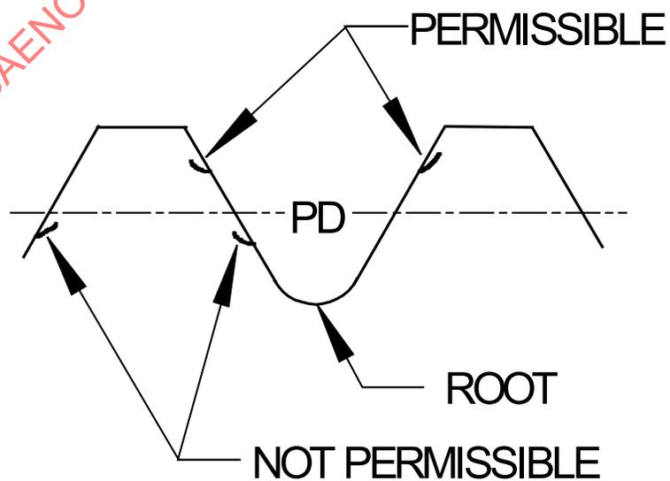
Figure 6 - Laps extending towards crest, rolled thread
