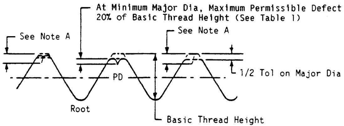
Note A: Depth of defect equals 20% of basic thread height plus 1/2 the difference of the actual major diameter and minimum major diameter.
