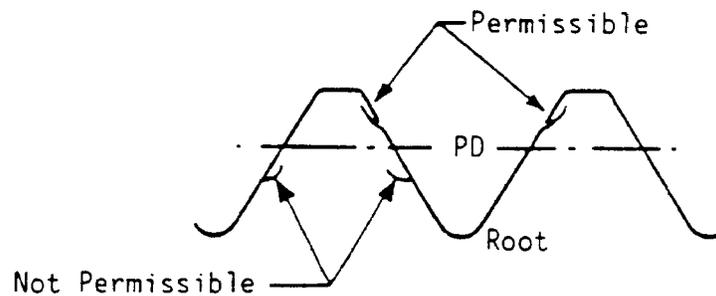
FIGURE 7 - LAPS EXTENDING TOWARDS CREST, ROLLED THREAD
