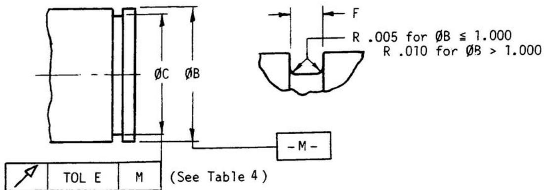
FIGURE 1 - Groove Dimensions, Type I, Classes 1 and 2 Retaining Rings
