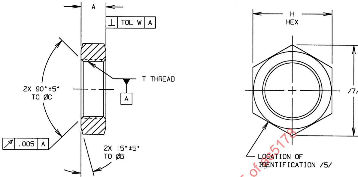
FIGURE 1 - FITTING, NUT
