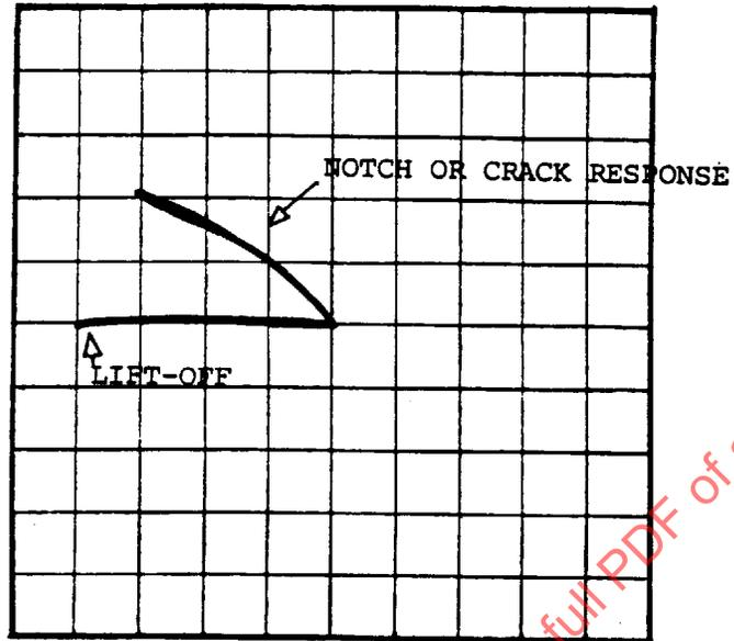
IMPEDANCE PLANE - NON-FILTERED DISPLAY AND ABSOLUTE DISPLAY
