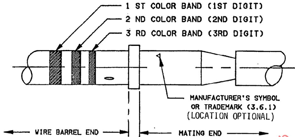
FIGURE 3 - CONTACT MARKING
