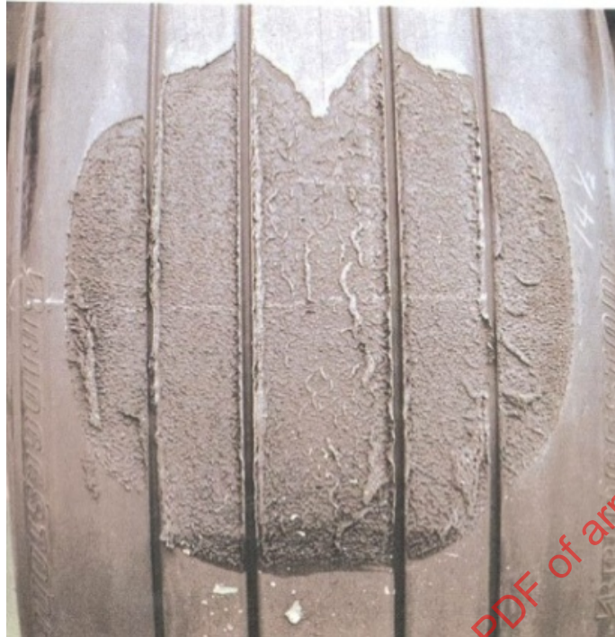
FIGURE 8 - TREAD RUBBER REVERSION
