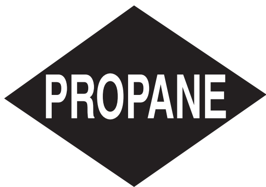
FIGURE 42.5.2.4 Example of Vehicle Identification Marking. [58:Figure 8.2.10]
