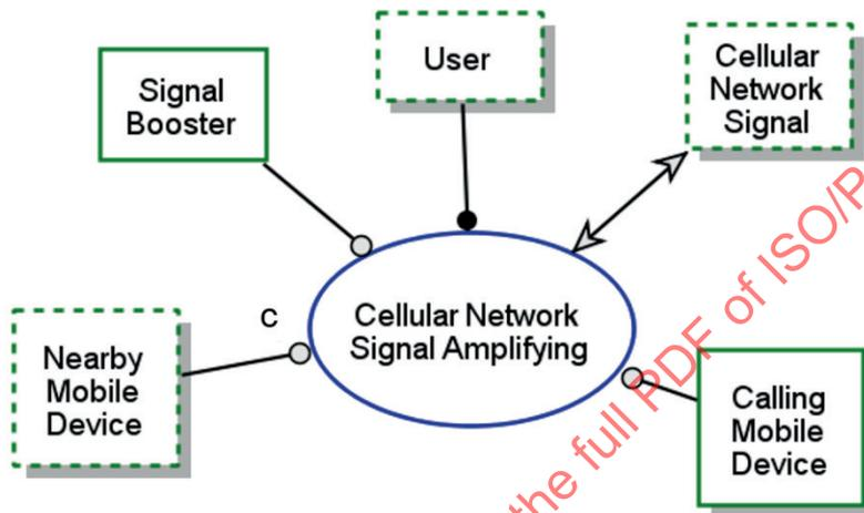
**Cellular Network Signal Amplifying** occurs if **Nearby Mobile Device** exists, otherwise **Cellular Network Signal Amplifying** is skipped.
