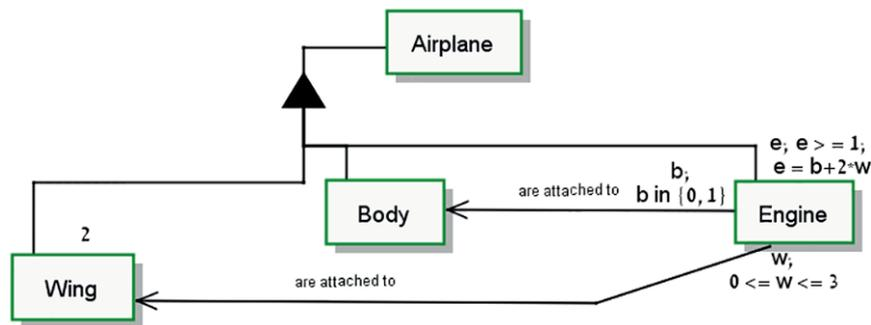
**Airplane** consists of **Body**, **2 Wings**, and **e Engines**, where  $e \geq 1$ ,  $e = b + 2 \cdot w$ .
