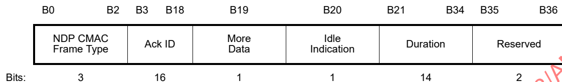
Figure 9-773—NDP CMAC frame body field of the NDP_2M PS-Poll-Ack frame
