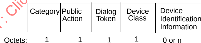
Figure 8-460i—GDD Enablement Request frame Action field format
