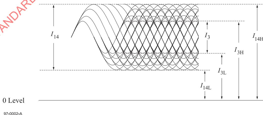
Figure 10 - Modulated amplitude
