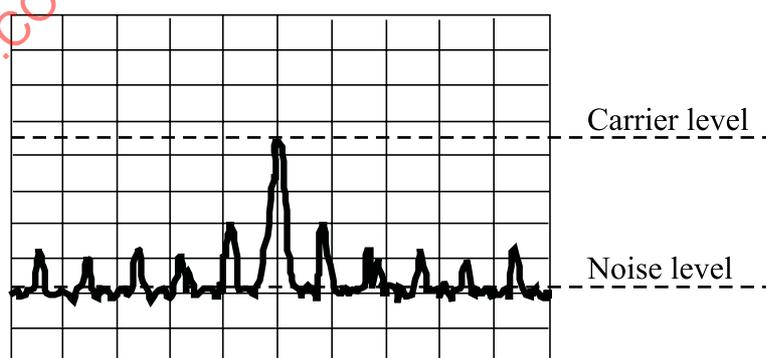
Figure 15 - Measurement of the wobble CNR
