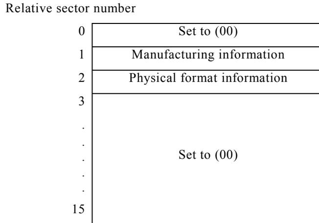
Figure 38 - Structure of a RW-Physical format information block
