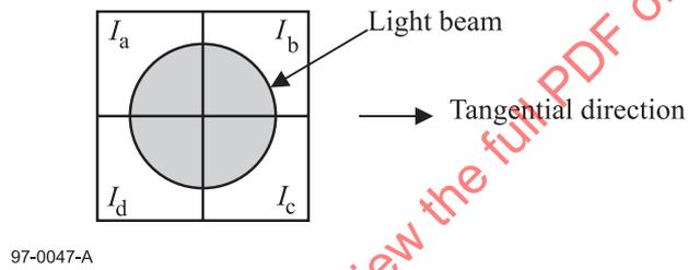
Figure 12 - Quadrant photo detector
