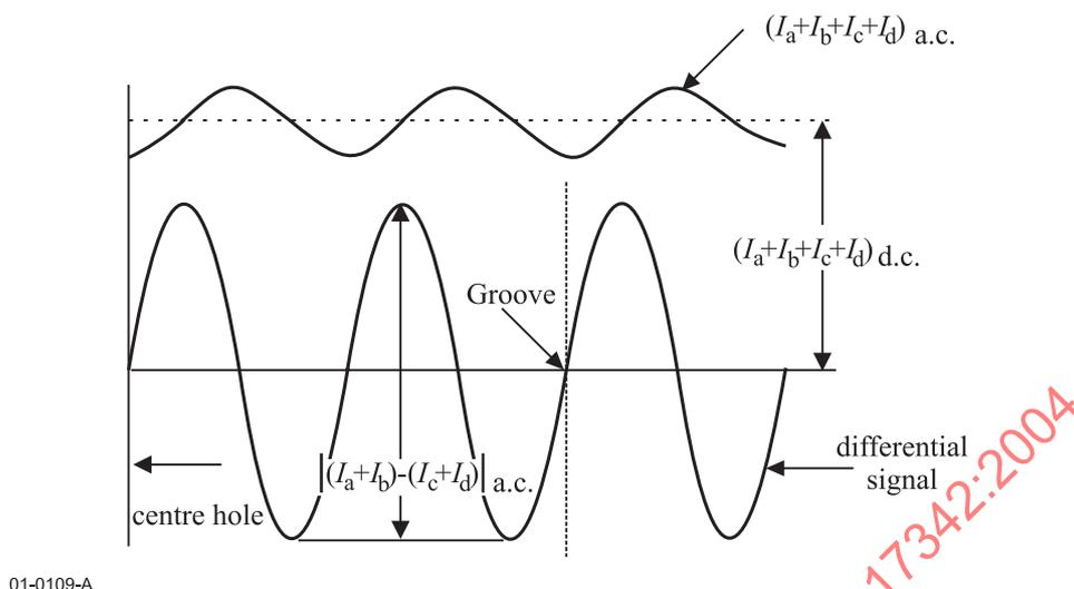
Figure 22 - Radial push-pull tracking error signal
