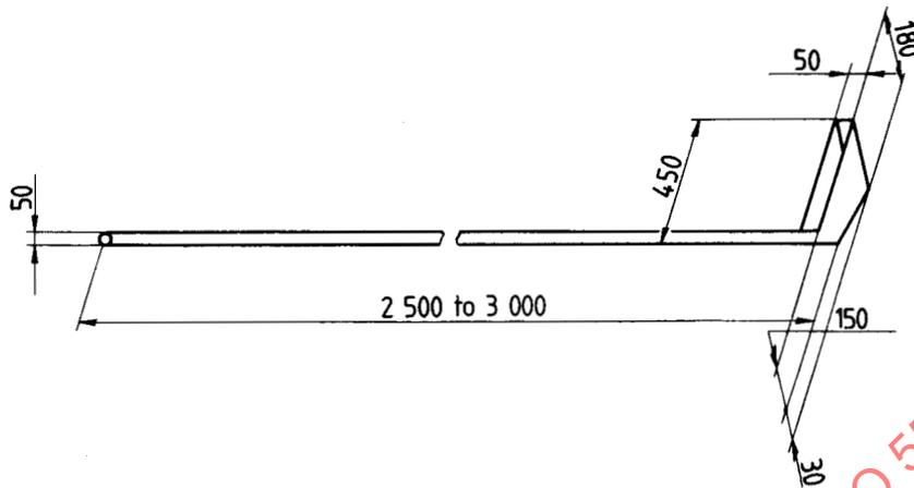
Figure 6 — Falling stream sampler (Pelican type)
