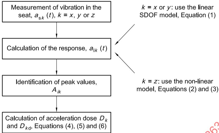
Figure 1 — Flowchart for acceleration dose calculation
