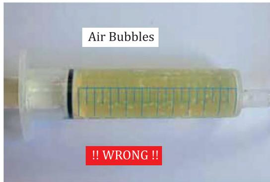
**Figure B.3 — Invalid sample with bubbles**
