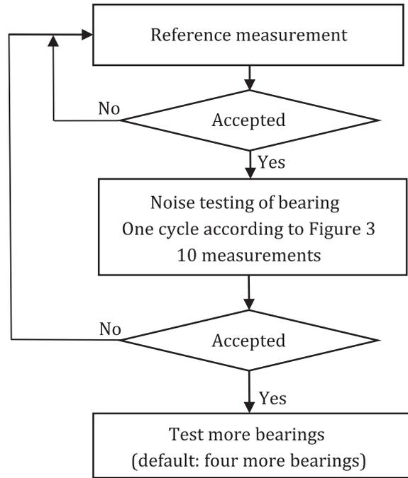
Figure 2 — Flow chart of grease noise assessing BQ+
