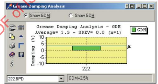
d) Bar chart, damping ability of the grease showing the  $GD_{MBQ+}$  value
