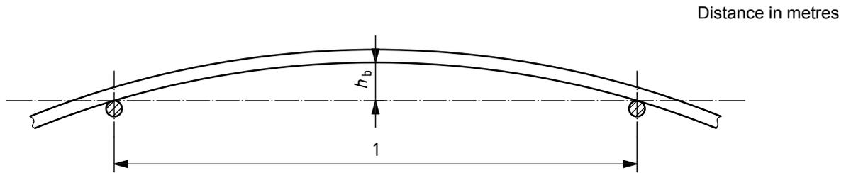
Figure 7 — Measurement of bow height
