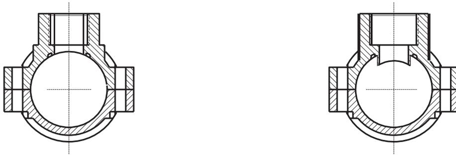
a) Without protrusion into the pipe
