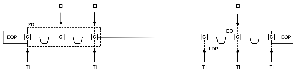
Figure 5a – Zone distribution cabling
