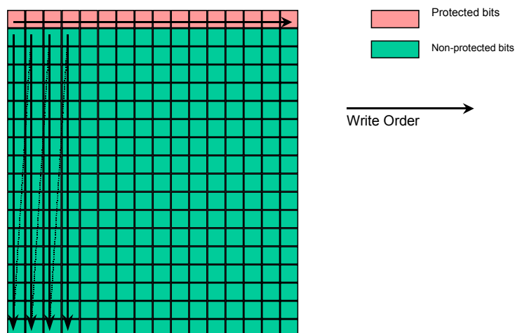
Figure 1.12 – One stage of interleaving
