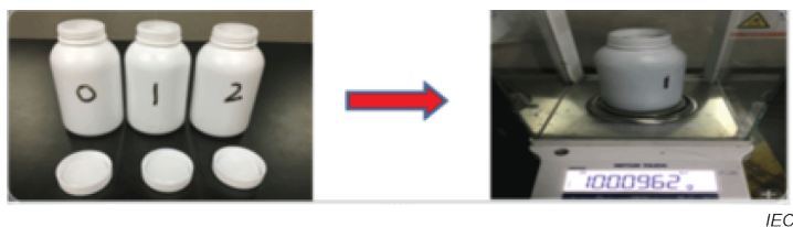
Figure C.2 – Procedure for weighing sample
