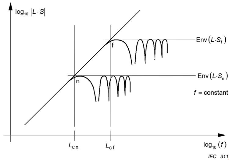
NOTE 1 For  $L > L_c$ , the maximum value of  $T$  is attained, i.e. the maximum coupling (or the screening attenuation) is not dependent on  $L$ .
