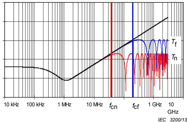
Figure 84 – Calculated coupling transfer function
