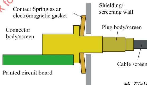
**Figure 63 – Cross-sectional sketch of a typical feed-through configuration**
