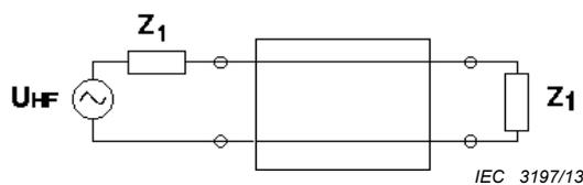
**Figure 81 – equivalent circuit of the set-up without DUT**
