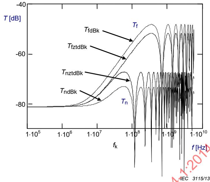
$T_f$  is 3,5 dB higher and  $T_n$  is 6 dB lower than in reference Figure 9 because
