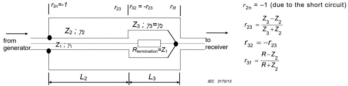
**Figure 58 – Triaxial set-up, impedance mismatches**
