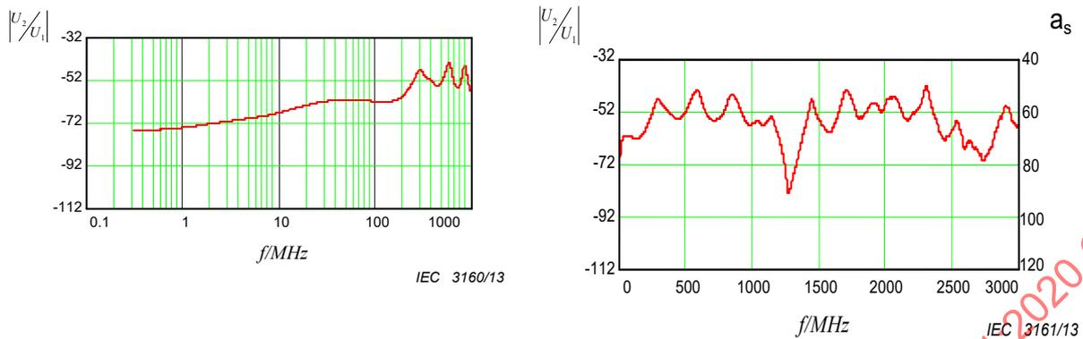
Logarithmic voltage ratio  $|U_2/U_1|$  in dB (left hand scale) and screening attenuation  $a_s$  (right hand scale)
