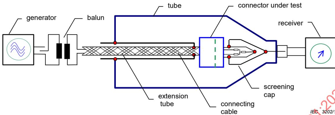
**NOTE** The balun transformer is not required in case of multiport VNA with mixed mode capabilities, see Annex A.
