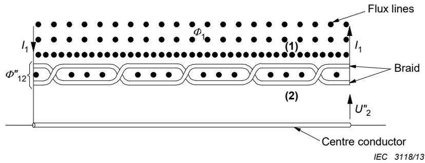
**Figure 14 – Magnetic coupling in the braid – Complete flux**
