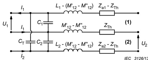
Figure 20b – Significant elements of circuits (1) and (2)
