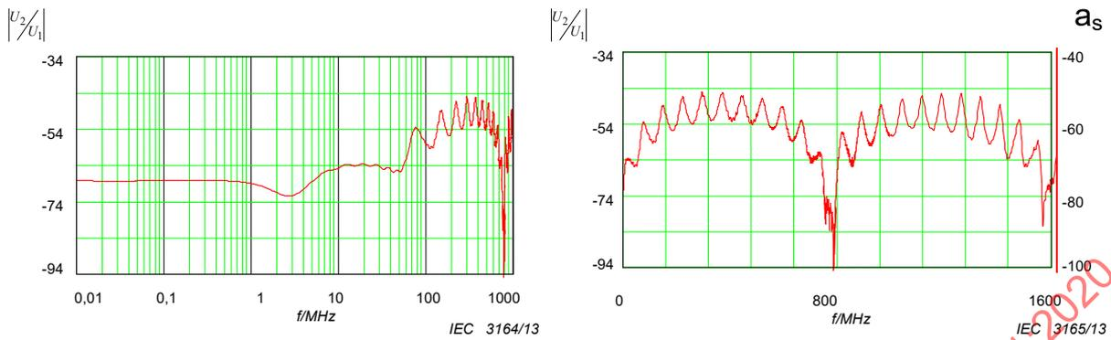
Logarithmic voltage ratio  $|U_2/U_1|$  in dB (left hand scale) and screening attenuation  $a_s$  (right hand scale),  $\epsilon_{r1}=1,7$ ,  $|\Delta v/v_1|=24\%$ , coupling length  $L = 2$  m.
