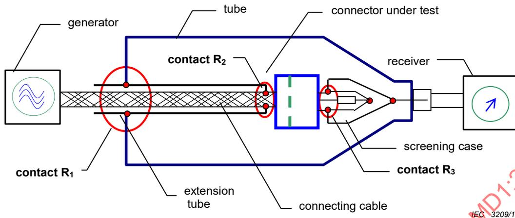
**Figure 91 – Contact resistances of the test set-up**
