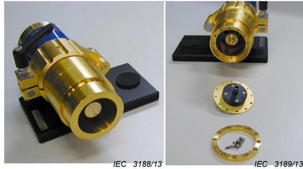
**Figure 75 – Detailed views of the contact area the test fixture and the secondary side of side opened**
