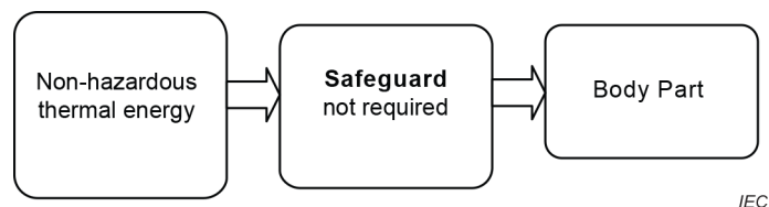
Figure 40 – Model for absence of a thermal hazard
