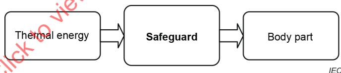
Figure 39 – Model for safeguards against thermal burn injury
