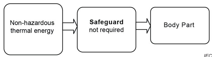
Figure 40 – Model for absence of a thermal hazard
