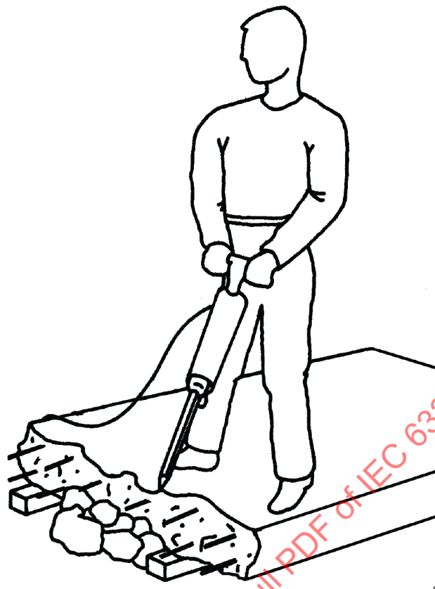
Figure 102 – Working position for percussion hammers and rotary hammers in percussion only mode (if applicable)
