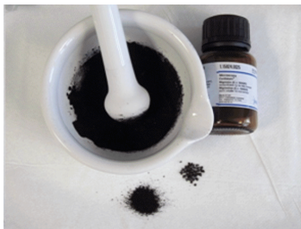
Figure 3 – Coarse Nigrosin kernels are ground in a chemical mortar
