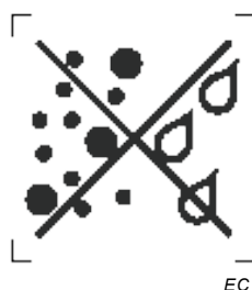
Figure 1 – Lamp not suitable for use under dust and moisture
