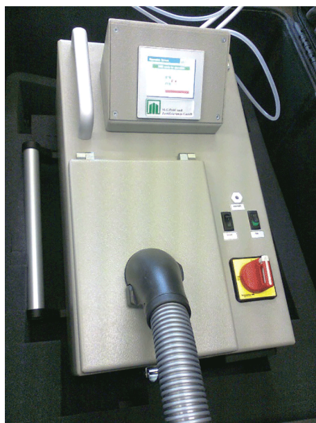
Figure C.1 – RSB with passive and active nozzle and vacuum measuring box
