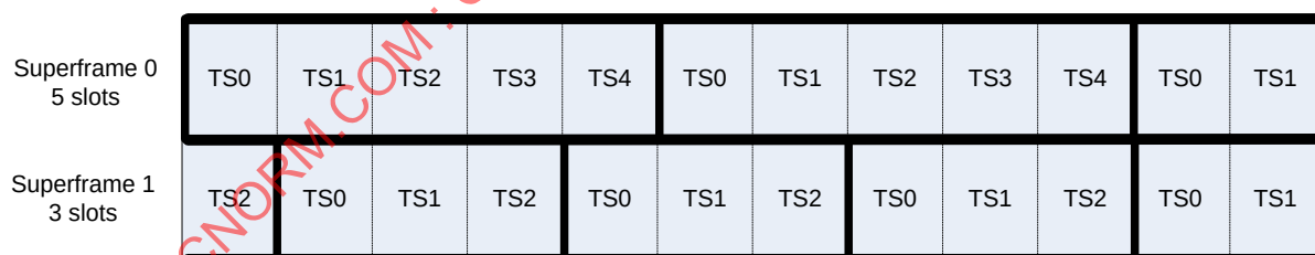
Figure 69 – Multiple superframes with aligned timeslots
