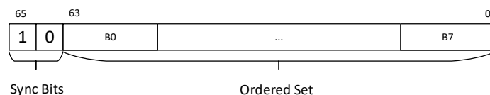
(a) Ordered Set Symbol structure in 64b/66b encoding
