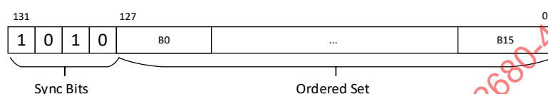
(b) Ordered Set Symbol structure in 128b/132b encoding
