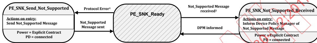
Figure 8-61 Sink Port Not Supported Message State Diagram
