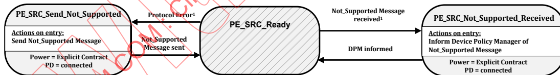
Figure 8-60 Source Port Not Supported Message State Diagram
