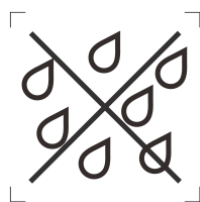
Figure 6 – Lamp not suitable for use under moisture
