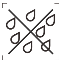
Figure 6 – Lamp not suitable for use under moisture
