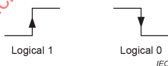
Figure 11 – Bi-phase encoded bits
