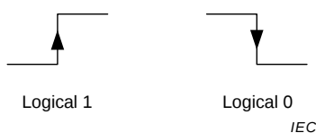
Figure 11 – Bi-phase encoded bits
