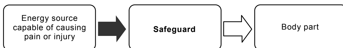
Figure 2 – Three block model for safety
