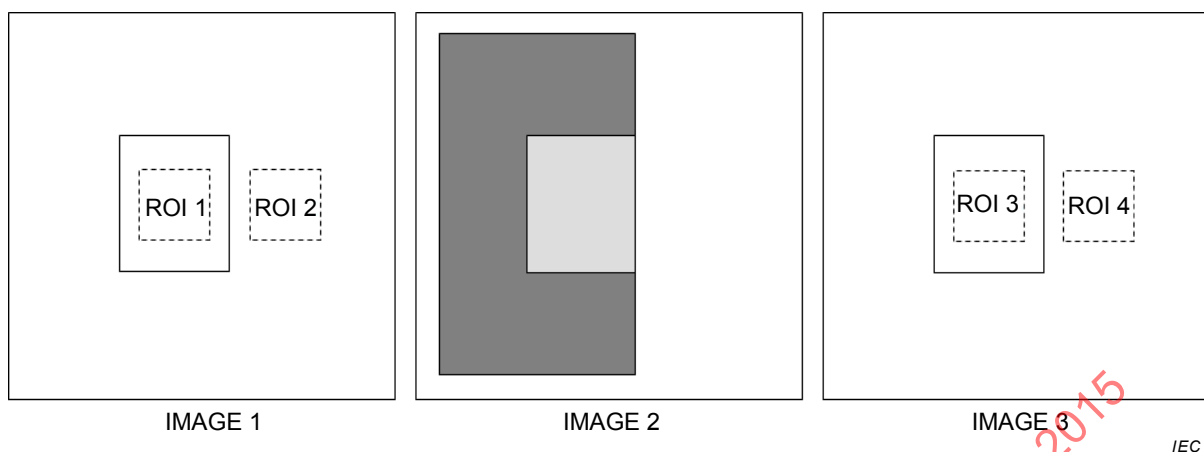
Figure A.3 – Definition of the ROIs for the test of the multiplicative LAG EFFECTS
