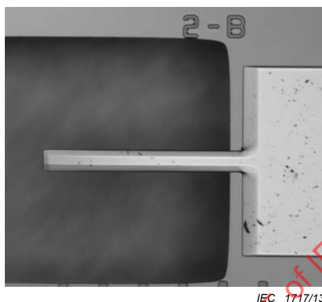
Figure B.1 – Cantilever type bend test piece of metallic glass in accordance with IEC 62047-18
