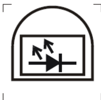
Figure 1 – Symbol for built-in LED modules
