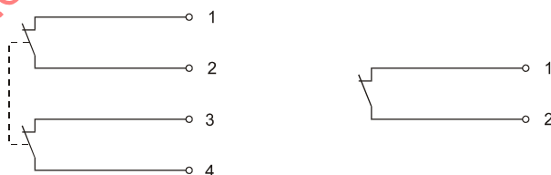
Figure A.7 – Connection of mechanical switches
