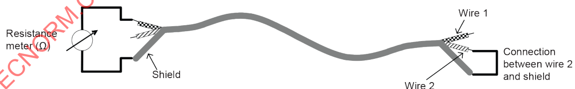
Figure N.4 – Resistance measurement for detecting wire shorts
