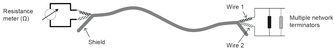
Figure N.5 – Resistance measurement between wire 1 and wire 2
