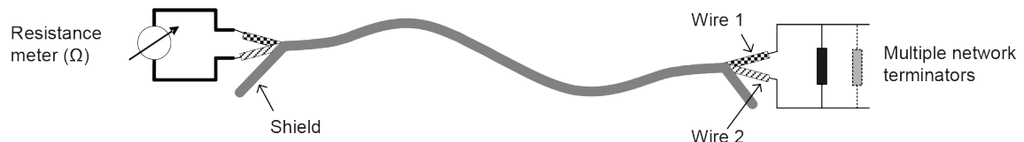
Figure N.5 – Resistance measurement between wire 1 and wire 2
