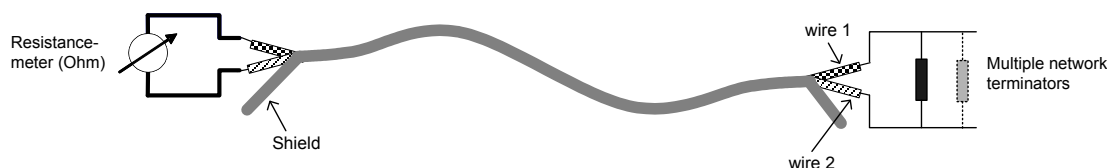
Figure N.5 – Resistance measurement between wire 1 and wire 2
