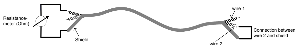
Figure N.4 – Resistance measurement for detecting wire shorts
