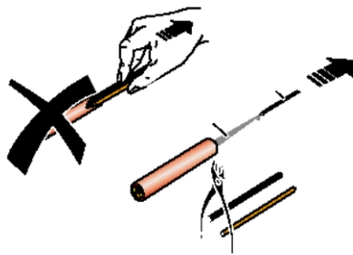
Figure 23 – Do not pull by the individual wires
