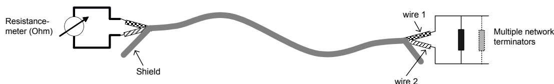
Figure N.5 – Resistance measurement between wire 1 and wire 2
