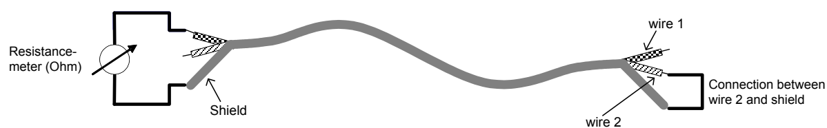
Figure N.4 – Resistance measurement for detecting wire shorts
