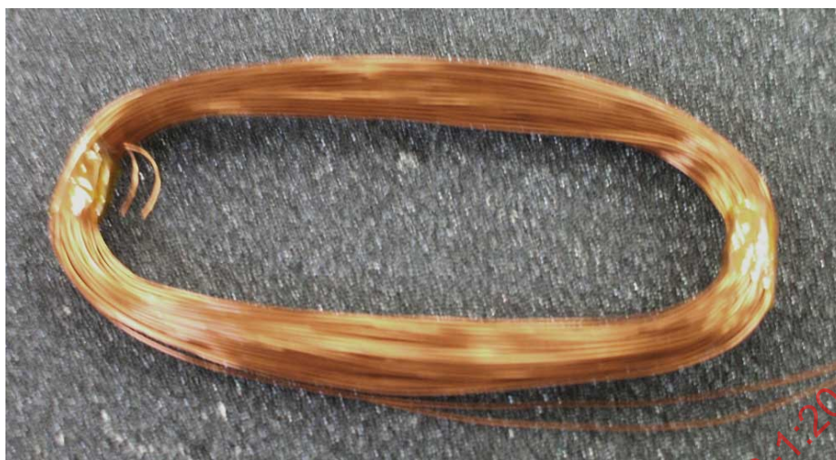
Figure B.7 – Example of random-wound coil
