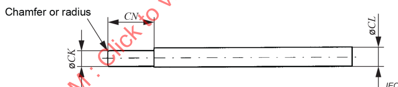
Figure 3 – Pin gauge for adaptor
