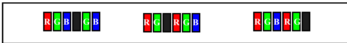
Figure 3 a) – One dark subpixel defect
