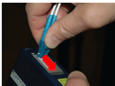
Figure D.6 – cleaning of cylindrical ferrule
