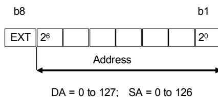
Figure 16 – Address octet coding
