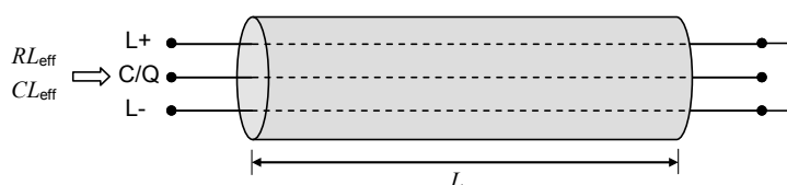
Figure 25 – Reference schematic for effective line capacitance and loop resistance
