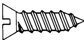
Figure 1 – Thread-forming tapping screw (3.6.10)
